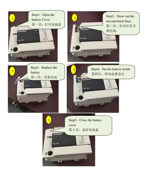
Attention: When the PLC voltage is low, Replacing the battery requires live replacement, Otherwise it is easy to lose the PLC program.
